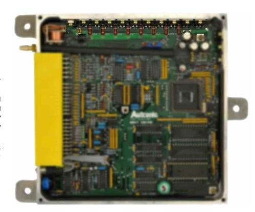
Late SM2 ECUs (Revs F & G) are fitted with current selectable switching type Injector Drivers. When a jumper link is fitted between pins 1 & 2 of CON3 drive current is high (4A peak / 1A hold). When a jumper link is fitted between pins 2 & 3 of CON3 drive current is low (2A peak / 0.5A hold). Last 2 characters of the serial number indicates the jumper selection fitted when the product left the factory ('A2' = 2Apeak / 0.5A hold, 'A4' = 4A peak / 1A hold).
