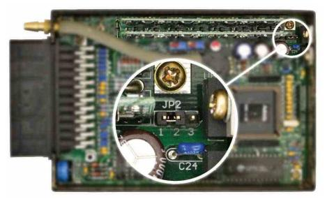
Late SMC ECUs (Revs D & E) are fitted with current selectable switching type Injector Drivers. When a jumper link is fitted between pins 1 & 2 of CON3 drive current is high (4A peak / 1A hold). When a jumper link is fitted between pins 2 & 3 of CON3 drive current is low (2A peak / 0.5A hold). Last 2 characters of the serial number indicates the jumper selection fitted when the product left the factory ('A2' = 2A peak / 0.5A hold, 'A4' = 4A peak / 1A hold).
