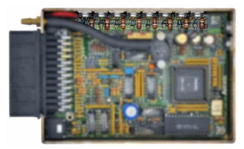
Early SMC ECUs (Revs A thru C) are fitted with fixed current Injector Drivers (attached to side of case). Last 2 characters of the serial number identify the factory fitted driver type ('A2' = low = 2A peak / 0.5A hold, 'A4' = high = 4A peak / 1A hold). Drive current cannot be changed in the field. Contact AUTRONIC about driver replacement.
