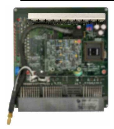
Early ECUs (Revs A & B) are fitted with fixed current Injector Drivers (attached to heatsink. Subaru ECU shown, EVO ECUs have same attachment). Drive current cannot be changed in the field. Contact
