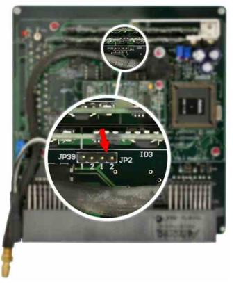
NOTE: This product is usually supplied with the correct drivers or driver jumpering to suit the OEM injectors of the intended application. Driver change or jumpering change may be required if non original injectors are installed
